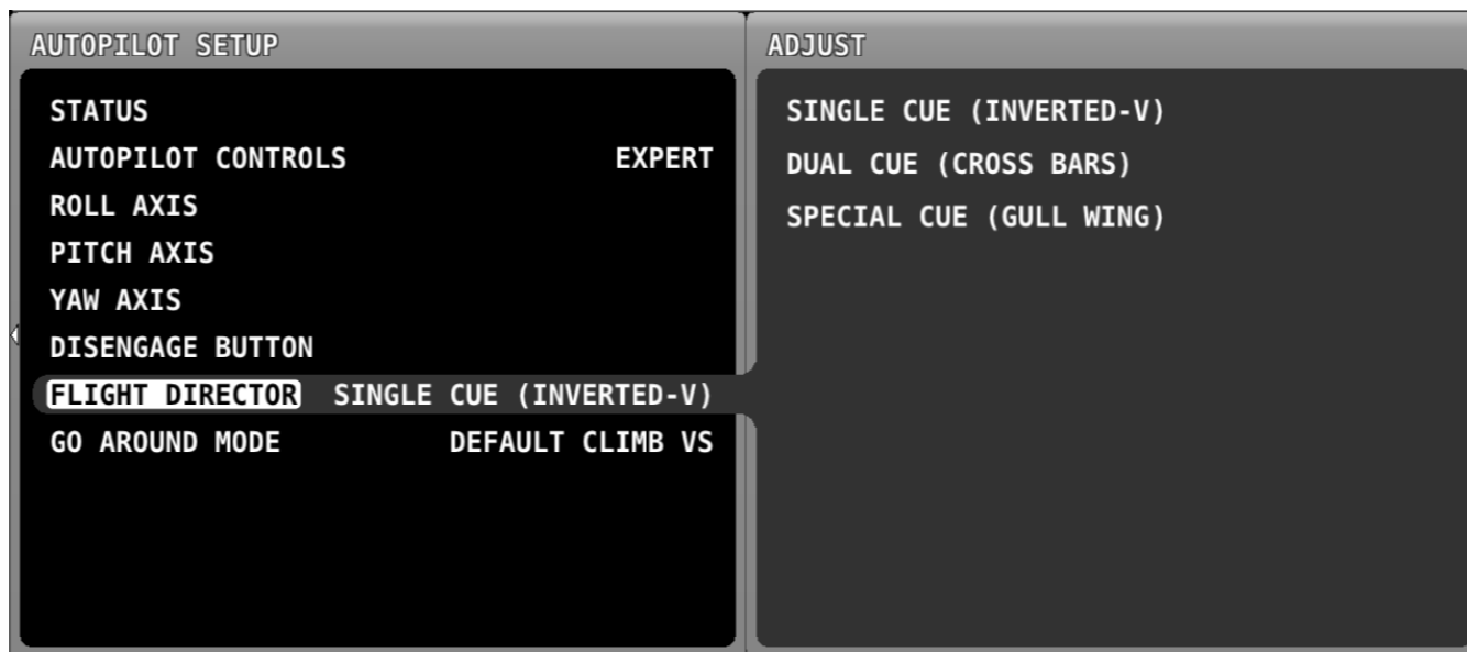
Figure 17 Flight Director Configuration
