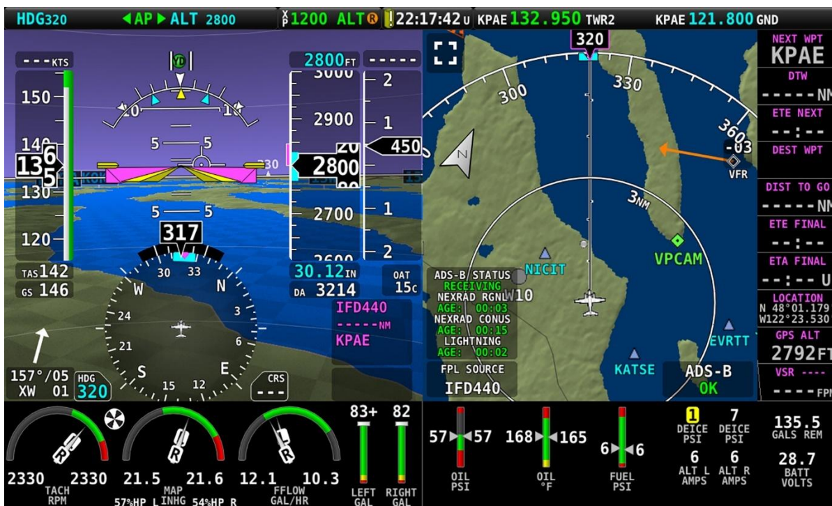
Figure 24: Example of Engine Bottom Band with PFD and MAP for Twin-engine Monitoring
