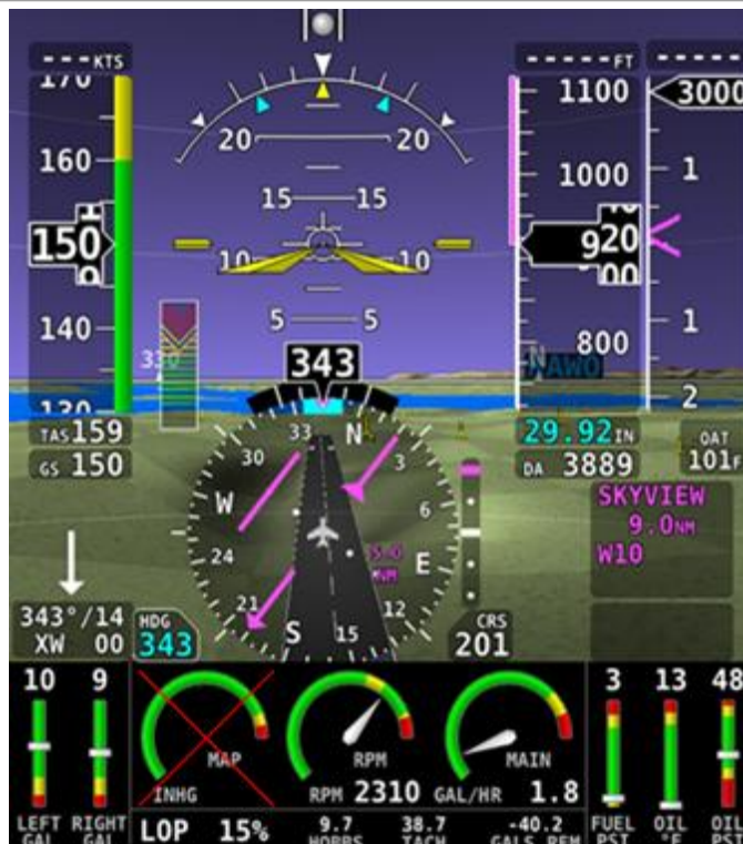
Figure 42: Example of an EMS Sensor Failure
