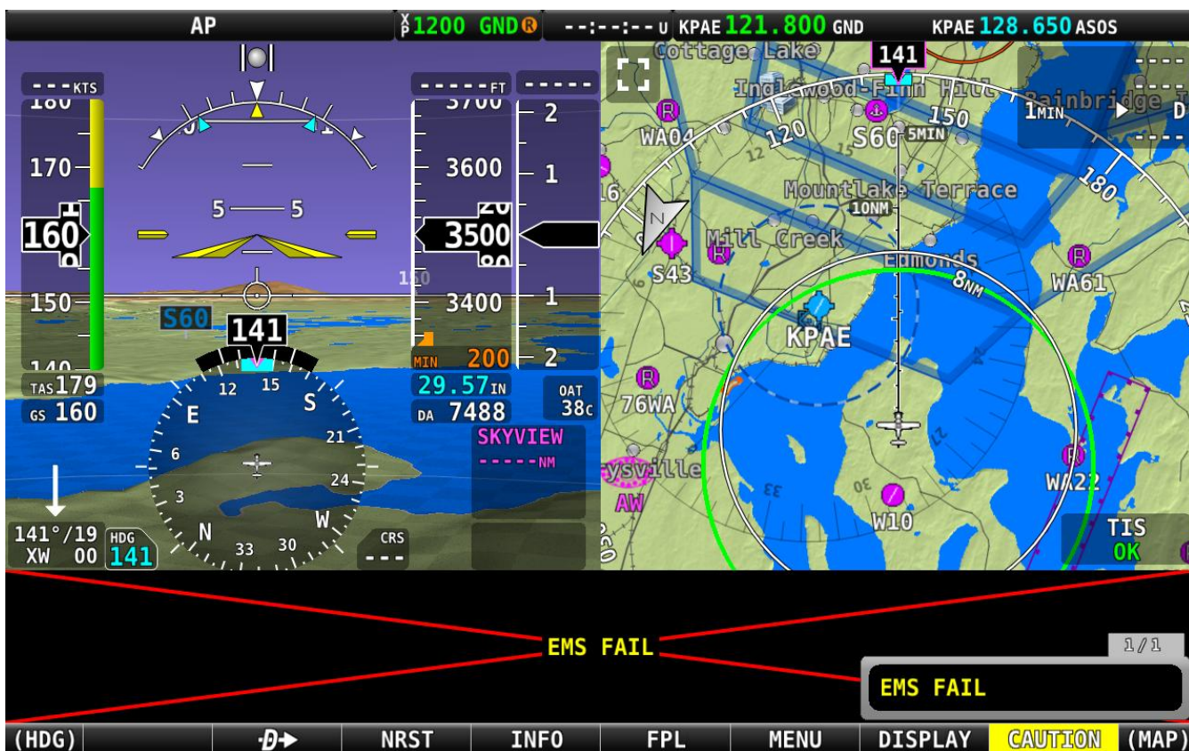
Figure 41: Example of EMS Module Failure
