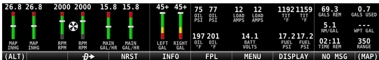
Figure 75 – Engine Bottom Band Layout for Twin-engine Monitoring
