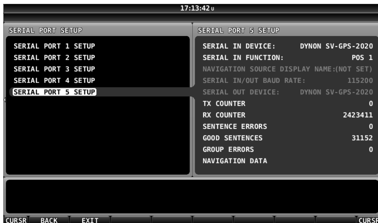
Figure 85: Serial Port 5 Setup for SV-GPS-2020
