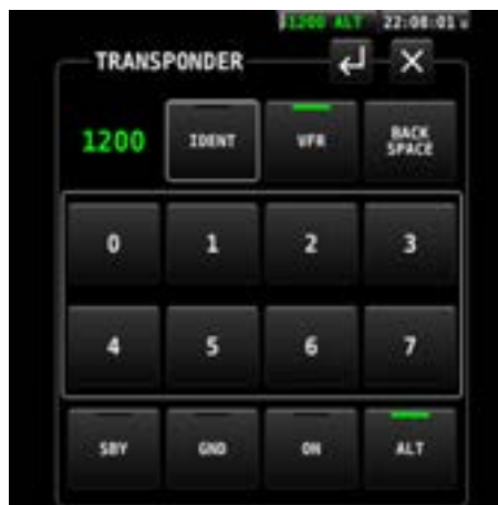
Mode S Transponder with 2020-compliant ADS-B Out
