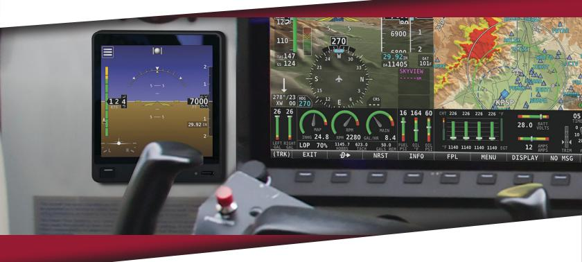
Meet the latest addition to the Dynon Certified product line: The Dynon D30 Touchscreen Electronic Flight Display. The D30 serves as a backup set of flight instruments in STC'd SkyView HDX systems\*, which can now be installed into over 600 type certificated aircraft models.
