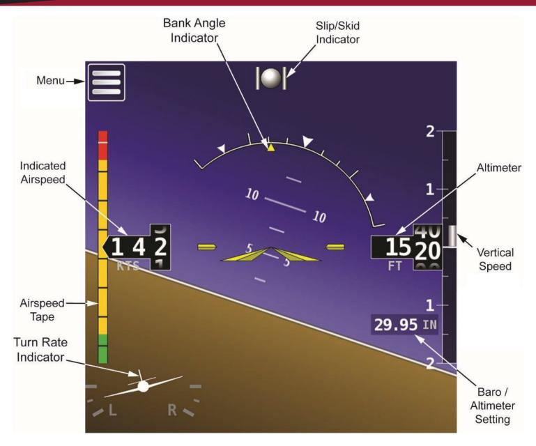
Featuring the largest, highest resolution sunlight readable display in its class, the D30 provides a crisp and clear view of critical backup flight information. The D30 is a robust set of backup instruments, including attitude, airspeed, altitude, vertical speed, turn rate, and slip/skid indications.
